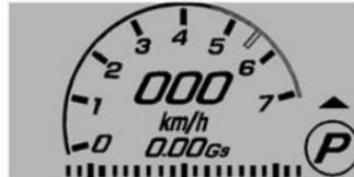
**Sport:** Displays the vehicle speed, a circular tachometer, shift indicator, and G-Force meter.
