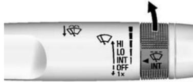
**INT (Intermittent Wipes):** Move the lever up to INT for intermittent wipes, then turn the
