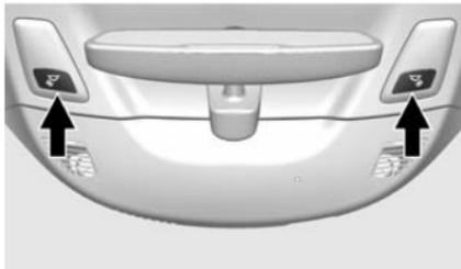
The reading lamps are in the overhead console. The lamps go on when a door is opened. When the doors are closed, press the lamp buttons to turn on each lamp.
