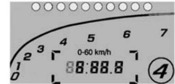
**Timing:** Displays a linear tachometer, gear position, shift lights, and performance or lap timer. The performance or lap timer content displayed depends on which feature is currently in use in the instrument cluster. See *Instrument Cluster* on page 5-8.
