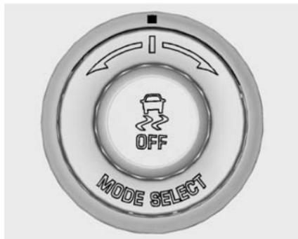
The TCS/StabiliTrak button is on the centre console.
