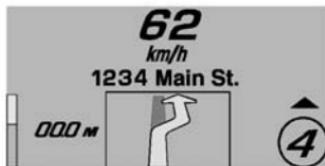
**Navigation:** Turn-by-turn navigation information may be displayed when Navigation is active and an upcoming manoeuvre is pending. It appears until the manoeuvre is complete and then the HUD display returns to the previous view.
