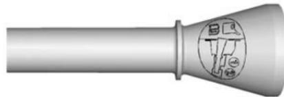
1. Locate the capless funnel adapter from inside the vehicle.
