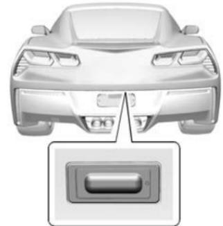
Press the release touch pad to open the boot if the RKE transmitter is within 1 m (3 ft).
