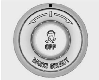
The Driver Mode Selector knob is on the console behind the gear lever.
