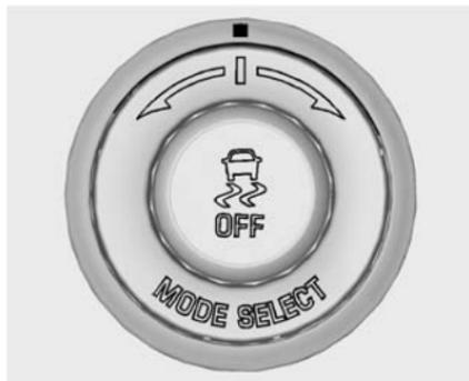
In order to select this optional handling mode, the vehicle mode must be Track. Then quickly press the TCS/StabiliTrak
