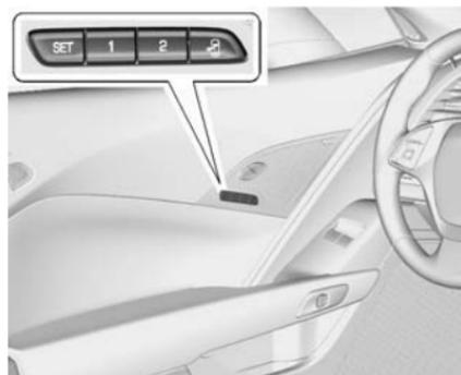
If equipped, the "1," "2," SET, and EXIT (Exit) buttons on the driver door are used to manually save and recall memory settings for the driver seat, outside mirrors, and power tilt and telescoping steering column.
