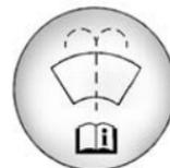
Open the cap with the washer symbol on it. Add washer fluid until the tank is full. See *Engine Compartment Overview* on page 10-7.
