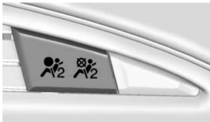
The passenger sensing system will turn off the front outboard passenger frontal airbag under certain conditions. No other airbag is affected by the passenger sensing system. See *Passenger Sensing System* on page 3-20.
