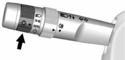
The exterior lamp control is on the indicator lever.
