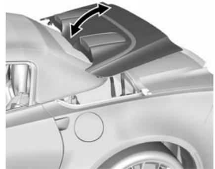
1. On each side of the tonneau cover, lift and pivot rearward into the fully open position.
