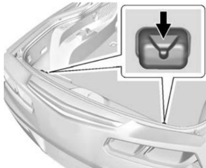
3. Line up the rear roof panel pins so that they drop into the receivers on the back of the storage area.
