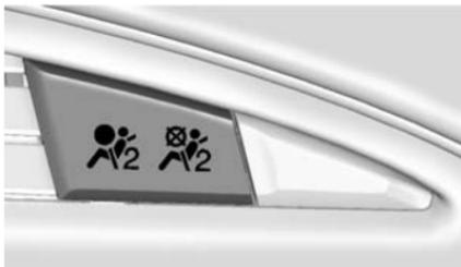
The symbol for on and off will be visible during the system check. When the system check is complete, either the symbol for on or off will be visible. See *Passenger Airbag Status Indicator on page 5-15*.
