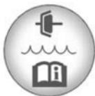
The hydraulic clutch fluid reservoir cap has this symbol on it. See *Engine Compartment Overview* on page 10-7 for reservoir location.
