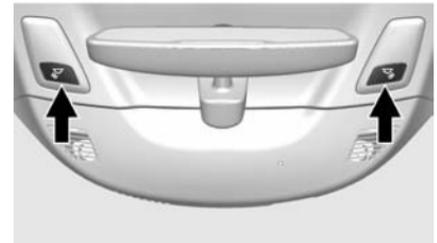
The reading lamps are in the overhead console. The lamps go on when a door is opened. When the doors are closed, press the lamp buttons to turn on each lamp.
