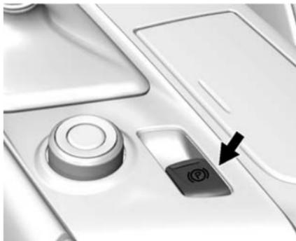
The vehicle has an Electric Parking Brake (EPB). The switch is on the centre console. The EPB can always be activated, even if the ignition is off. To prevent draining the battery, avoid repeated cycles of the EPB when the engine is not running.
