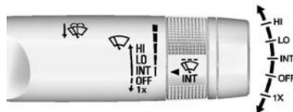
The window wiper/washer lever is on the right side of the steering column.
