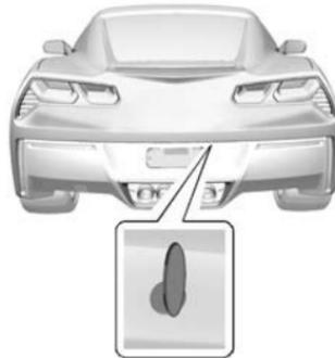
From outside the vehicle, use the key to open the hatch/boot. See *Keys* on page 2-1.
