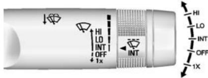
The windscreen wiper/washer lever is on the right side of the steering column.
