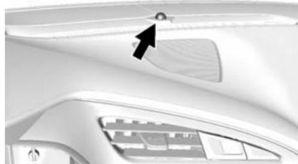
There is a light sensor on top of the instrument panel. Do not cover the sensor; otherwise the headlamps will come on when they are not needed.
