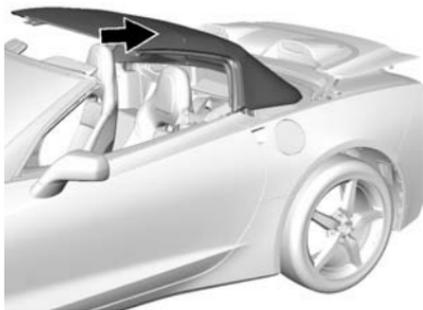
2. Lift and pivot the convertible top rearward into the fully stowed position.
