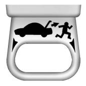
There is a glow-in-the-dark emergency boot release handle on the boot lid. This handle will glow following exposure to light. Pull the release handle to open the boot from the inside.
