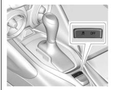
This optional handling mode can be selected by pressing the TCS/ StabiliTrak button two times. The appropriate message displays in the Driver Information Centre (DIC).
