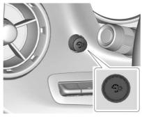
The knob for this feature is on the left side of the instrument panel.
