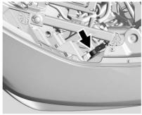
Locate the indicator socket bulb on the inboard side of the lamp.
