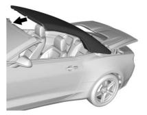
Lift and move the convertible top forward by pulling on both sides of the front bow into the fully closed position.
