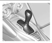
DSC allows shifting an automatic transmission similar to a manual gearbox. To use the DSC feature:
