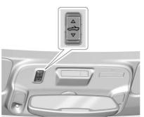
After the convertible top is completely open, a Driver Information Centre (DIC) message displays. Release the switch.
