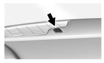
The vehicle has a light sensor on the top of the instrument panel. Do not cover this sensor, otherwise the system will come on whenever the ignition is on.
