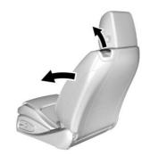
To access the rear seats, pull up on the latch on the top of the driver or front passenger backrest. Fold the backrest forward.
