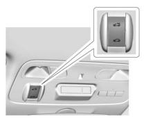
If equipped, the sunroof only operates when the ignition is on or in ACC/ACCESSORY, or when Retained Accessory Power (RAP) is active. See Retained Accessory Power (RAP) ⇒ 169.
