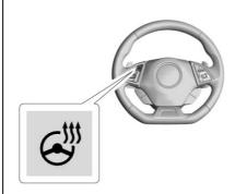
Press to turn the heated steering wheel on or off. A light next to the button displays when the feature is turned on. The steering wheel takes about three minutes to be fully heated.
