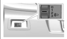
The manual headlamp levelling control is on the outboard side of the steering column. This feature lets the headlamp level be adjusted
