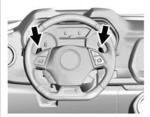
Tap Shift allows you to manually control the automatic transmission. To use Tap Shift, the gear lever must be in DSC mode. Vehicles with this feature have indicators on the steering wheel. The paddles are on the back of the steering wheel. Tap the left paddle (-) to downshift, and the right paddle (+) to upshift. The Driver Information Centre (DIC) display indicates the gear the vehicle is in.
